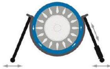
Hydraulic chest-lifting system
